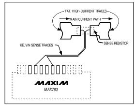
Figure 5. Kelvin Connections for the Current-Sense Resistors
