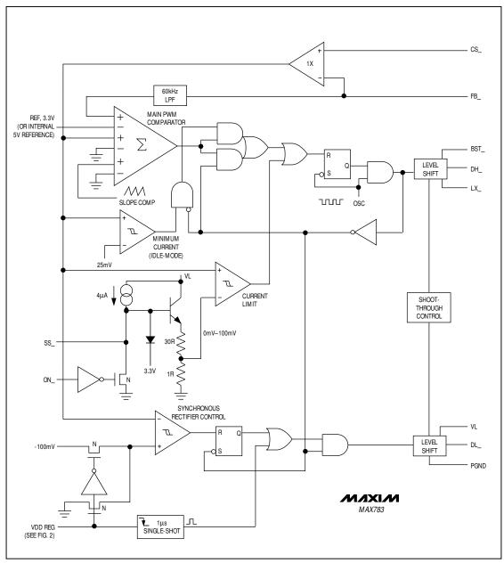
Figure 3. PWM Controller Block Diagram
