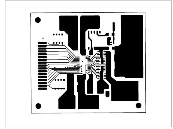
Figure 9. MAX783 EV Kit Top Layer (Layer 1), Top View
