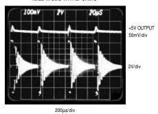
I<sub>LOAD</sub> = 100mA V<sub>IN</sub> = 10V
