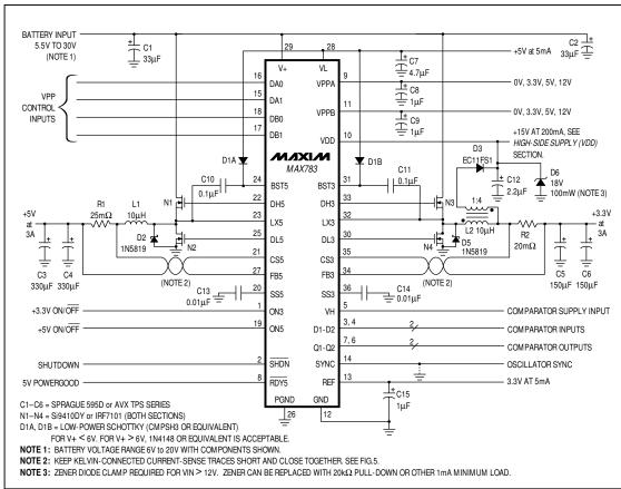
Figure 1. Standard Application Circuit
