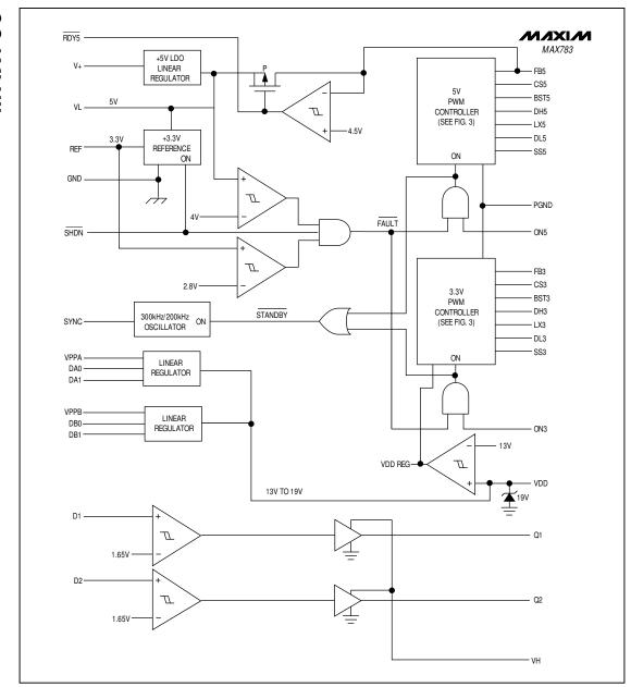
Figure 2. Block Diagram
