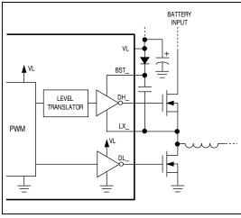
Figure 4. Boost Supply for Gate Drivers
