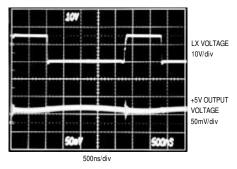
$I_{LOAD} = 1A$  $V_{IN} = 16V$
